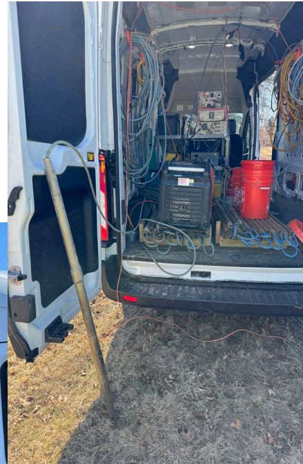
Deployment of a membrane interface hydraulic profiling tool (MIHPT) along Tozer Rd to collect groundwater data (March 2023)
