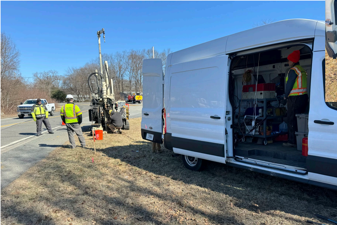
Deployment of a membrane interface hydraulic profiling tool (MIHPT) along Tozer Rd to collect groundwater data (March 2023)
