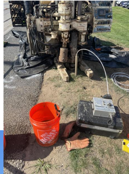
Collecting groundwater sample along Tozer Road via DPT drilling (August 2024)
