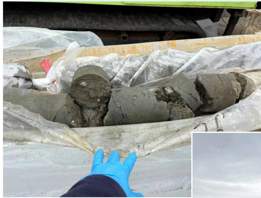
Dense glacial till from beneath Building 5 (5 to 55 ft deep)
