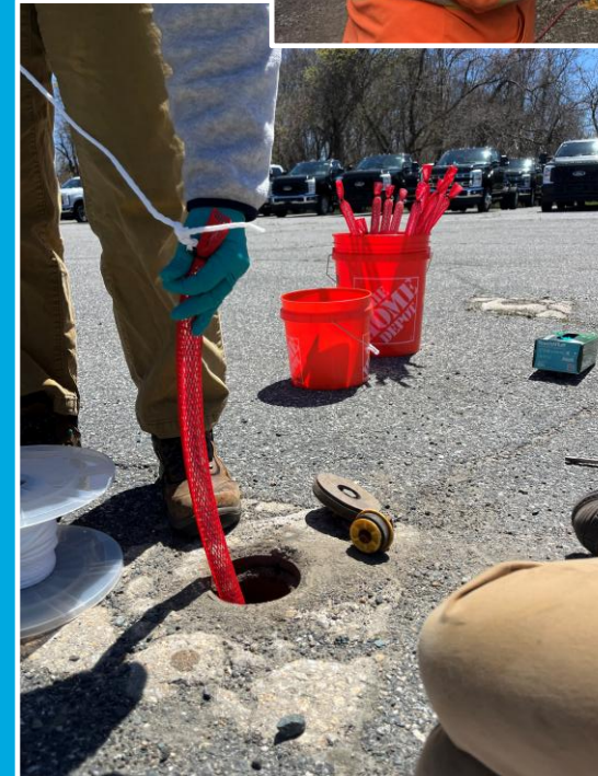
Deploying sampling equipment into monitoring wells
